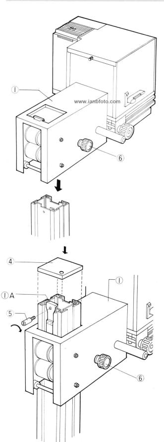
Loosen the carriage lock knob (6) by turning it counter-clockwise. Lift the entire head assembly as shown, matching the column and the opening of the carriage, and put the assembly over the column.
