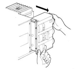
Let the module slide forward as shown, off the lamphouse.
