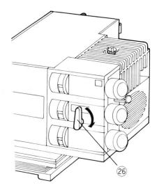
The white-light-focus lever (26), when turned to horizontal position, takes the filters out of the light-path without changing the set values, for easy focusing.
