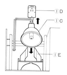
Pull the lamp socket (1D) out of the chamber. Put the enlarging-lamp (1C) in the socket, and put the lamp in the lamp-holder frame (1E) inside the chamber as shown.
