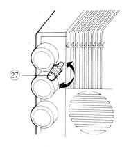
The light attenuator knob (27), when turned fully clockwise, brings the attenuator into the light-path, reducing the light to approximately 1/4 (two f-stops). Use it to extend exposure time when desired.
