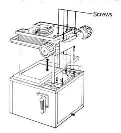
Place the head assembly upsidedown and loosen the four screws with the screwdriver.
